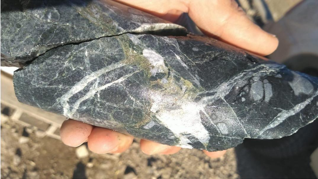
**Figure 3 – 19VNDD001 (299.6m). Mineralisation as blebs and disseminated grains of pyrite and chalcopyrite associated with coarse-grained epidote and calcite**
